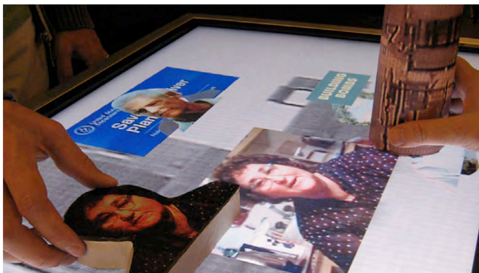
Figure 2. As KinoPuzzle tangibles are brought together, video clips are triggered on the table surface
