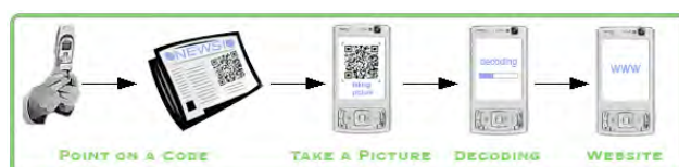
Figure 2. Mobile tagging process (source: Mobile tagging Blog, 2007)
