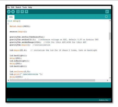
Fig.13: Sketch of data reading from the TDS Sensor
