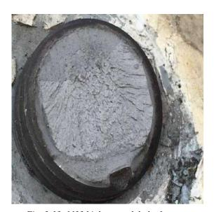
Fig. 3-13: M33 high strength bolts fracture
