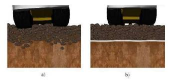
Fig.3: Simulation of geosynthetic application Source: LOPES (2005) apud FERREIRA (2010).
