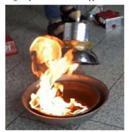
Fig. 1: Sound Fire Extinguisher from SSERI
