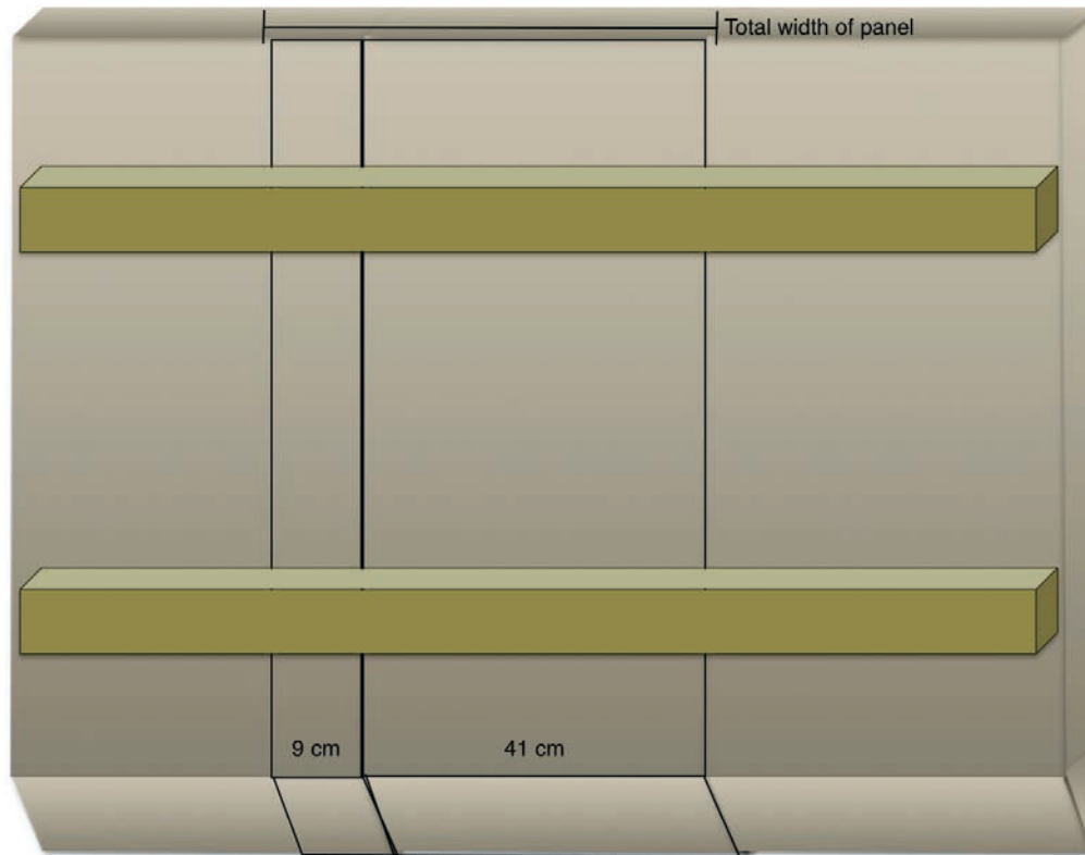
FIGURE 3. Diagram showing the possible construction of the panel support. Three or more boards of even width are joined together using crossbeams. The panel of St. John the Evangelist has been cut out of a section like this and consists of two boards 9 and 41 cm in width.
