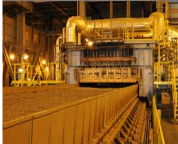
The easy to maintain sidewalls ensure that the feedstock remains on the pallet car. Our pallet cars are used in sintering machines with reaction areas up to 600 m 2 , with a grate factor of up to 45 tons of sinter per day and m 2 . Sinter bed heights up to 730 mm can be realized.
