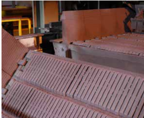
Metso Outotec pallet cars are used in pelletizing furnaces with reaction areas from 180 to 816 m 2 and with a grate factor of up to 28 tons of pellets per day and m 2 for hematite and 40 tons per day and m 2 for magnetite ores.
