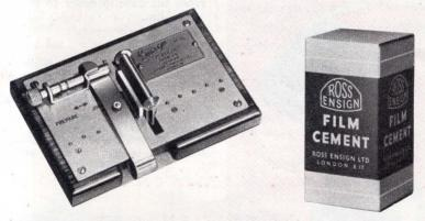
**POPULAR MODEL.** An inexpensive splicer which is ideal for those who edit only one size of cine film. It is supplied in any of the three narrow-gauge sizes—8 mm., 9.5 mm. or 16 mm.—and is provided with a built-in scraper accurately set for preparing the film. With the special Ross Ensign rapid-drying cement, neat, accurate joins can be made in a matter of seconds.
